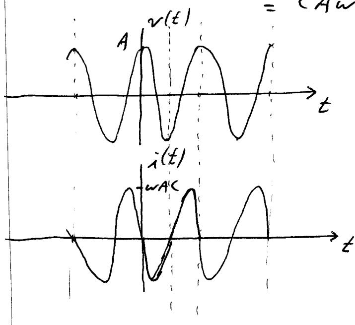
(Current is scaled in amplitude by factor  $\omega AC$ , and shifted in phase by  $90^\circ$ , relative to voltage.)
