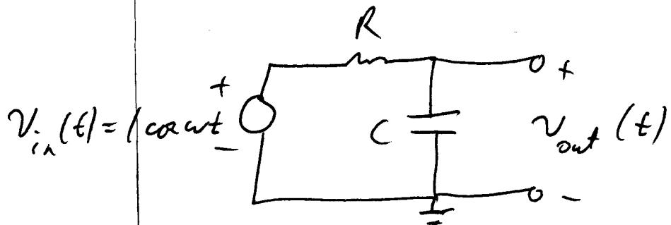
Redraw circuit with phasors + impedances - we will then be able to solve for the output voltage phasor, for a given input freq.  $\omega$ .
